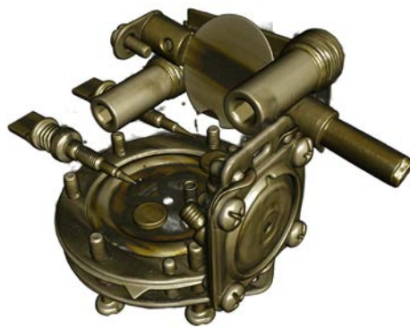
Figure 1 : Neutron tomography view of a carburetor (neither a CAD drawing nor a photo): metallic structures can very well be inspected with neutrons due to their high penetration and the high linearity in the attenuation coefficients
