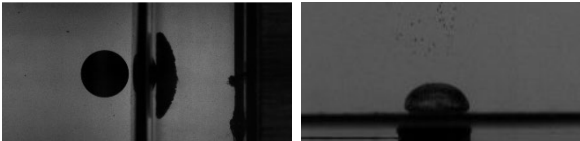
Figure: On the left, bubble produced by a steel ball (diam. 14 mm) launched by a gas gun at 50 m/s on a sandwich of stainless-steel plate (2 mm), water (3 cm) and PMMA (3 cm). On the right, cavitation due to laser shock on aluminium 0.8 mm plate confined with water, the impact is coming from the bottom.
