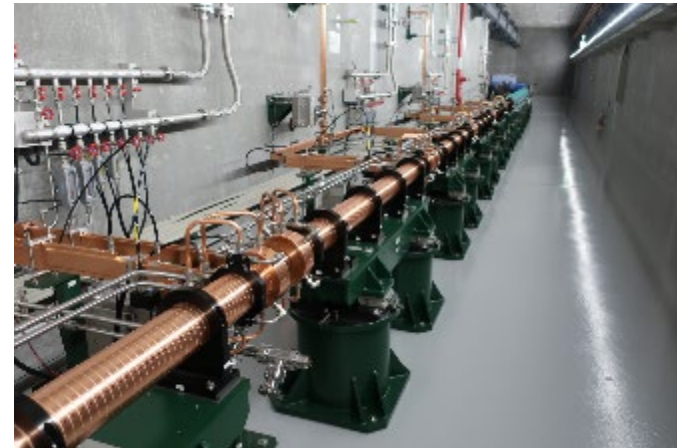
3 GeV C-band (5.7 GHz) accelerator (40 of 2m-long-cavities)
