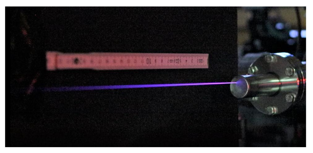
In the experimental hall at the European XFEL: The X-ray laser beam of 2.66 keV photons comes from the right, drills though the 2mm steel cap and generates a violet light phenomenon
