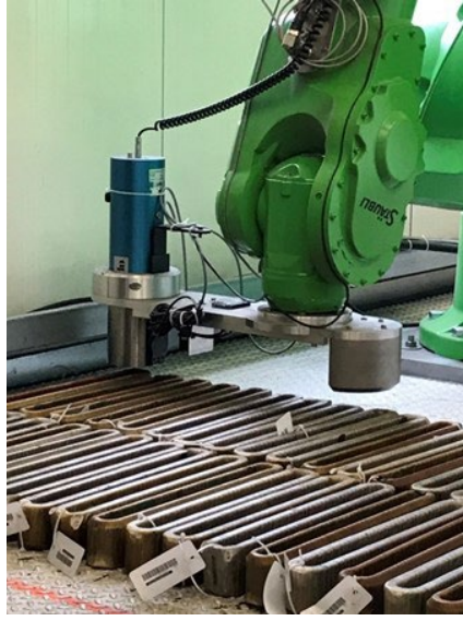
Robotised measurements of accelerator components in the ESRF-12 building
