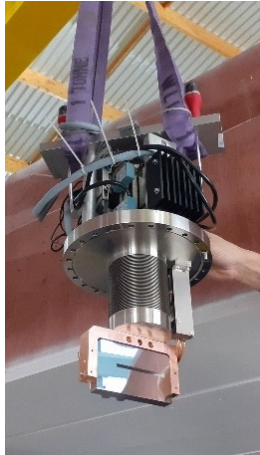
Slit mirror for the diagnostics beamline Test bed for new diagnostics in the frame of the upgrade
