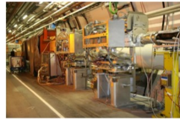
LHC Collimators and view of inside/jaws
