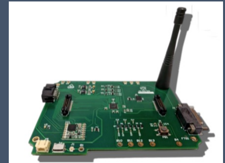
Radiation tolerant IoT hardware platform developed at CERN
