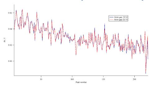
Step scan reduces vertical oscillation of probe but some position differences remain -> look at peak field only
