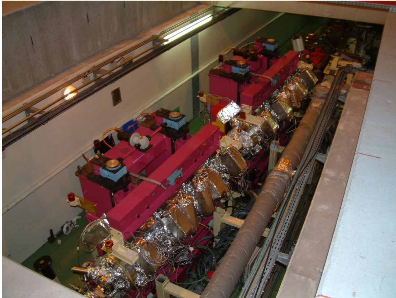
Two U23 in vacuum undulators of ID27
