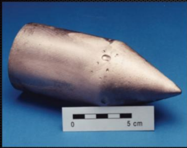
Heusler ( \text{Cu}_2\text{MnAl} ) polarising crystal (ILL)
