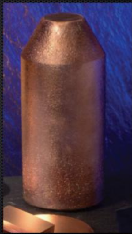
\text{\O}80 \times 300 \text{ mm}^3 Cu crystal (ILL)
