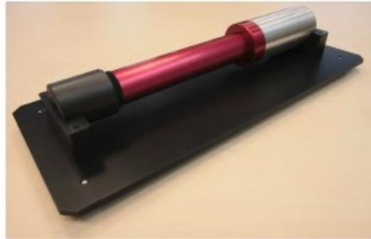
Test unit for scintillator test. The black cap houses beta source ( $Sr^{90}$ )
