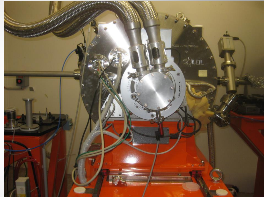
Galaxies DCM installed on the beamline
