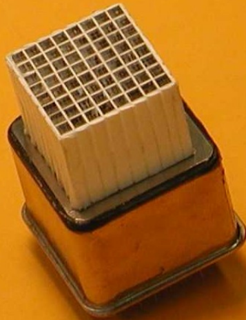
LYSO-LuYAP crystal matrix 2 x 2 x 10 mm 3
