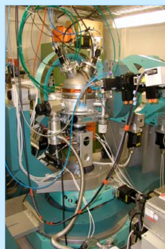
Diffractometer of beamline BM20 at the ESRF (ROBL-CRG) and perspective views of the sputter deposition chamber.
