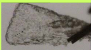
Optical micrograph of sample LCO1B2. The arrow indicates the position of the grain, less than 5 microns in size. The entrance track is optically visible and measures ~ 200 \mu\text{m} long and 50 \mu\text{m} large.
