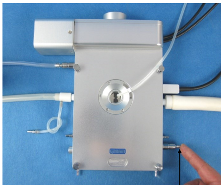
Block and release outlet valve with finger
