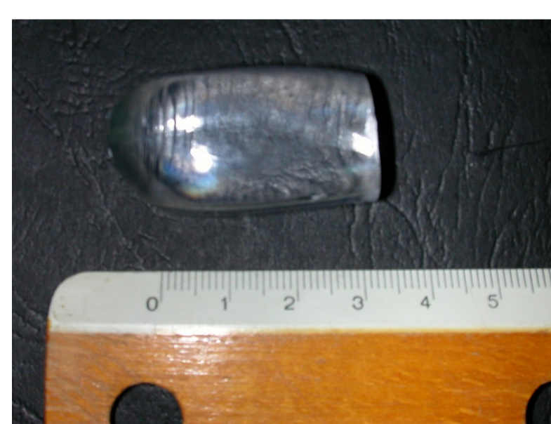
LiF monocrystal doped with 300 mg PbF_2 in melt
