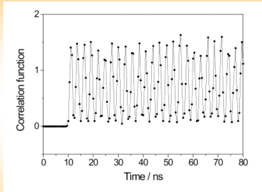
Continuous filling mode with 992 bunches equally spaced at 2.8 ns.
