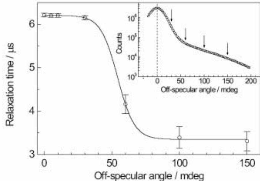
Off-specular:  $\tau = 3.3 \mu\text{s} \rightarrow$  homodyne detection.
