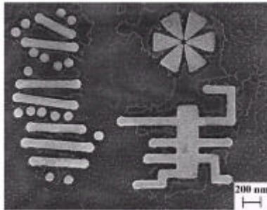
SEM image of sample Au nanostructured pattern (2.5 \mu\text{m} \times 2.0 \mu\text{m} )
