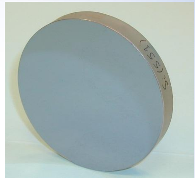
Spherically bent R=1 m Si551 crystal Credit: Roberto Verbeni (ESRF)
