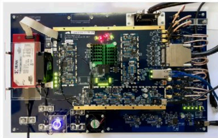
Hardware testing harness for FalconX hardware
