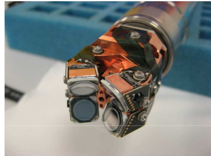
4 x 30 mm 2 SDD arrangement for TEM (top and bottom view on sample)
