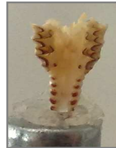
Head of a red tooth sore 1:1 capillary Source: Rh-Microfocus tube ( U=40\text{keV} , I=700\mu\text{A} ) Measurement time: 60min
