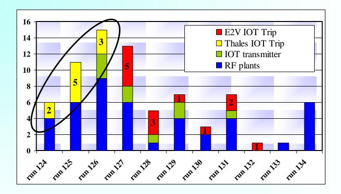
From 2010: number of RF plants failure and comparison between machine operation with Thales tubes (TH 793 and TH 793-1) and E2V tube D2130.
