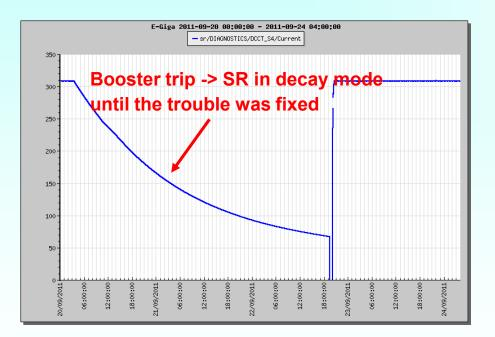
DECAY MODE: the RF cavity working point shifts according to the stored current. RF POWER  $\Delta$ ~1db, tuning  $\Delta$ ~10%.
