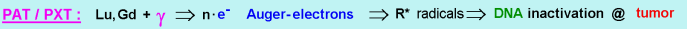
Fig.1: Photon activation therapy PAT (PXT) inactivates cancer cells by secondary radiation products after specific absorption of synchrotron X-ray photons at the K-edge of the target material.
