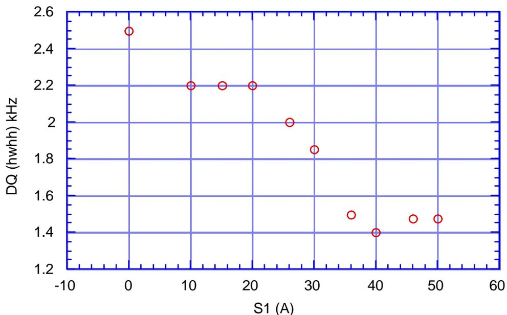
necessary damping and the effect is cancelled. In the graph above the tune incoherent frequency spread measured as a function of the S1 harmonic sextupole current for the multibunch case is shown. The optimum (for dynamic aperture) setting was 45 A whereas to damp, a 30 A setting was used. Possibly the the rate of the “instability” could be  $\sim 2\pi$  kHz
