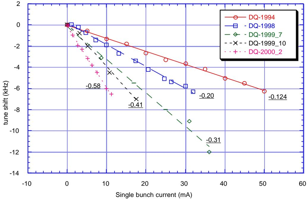
It is quite interesting to observe that the vertical effective impedance increases proportionally with the number of low gap chambers, i.e. each chamber adds about  $\sim 0.1$  kHz/mA to the original  $r_1 = 0.12$  kHz/mA. Since:
