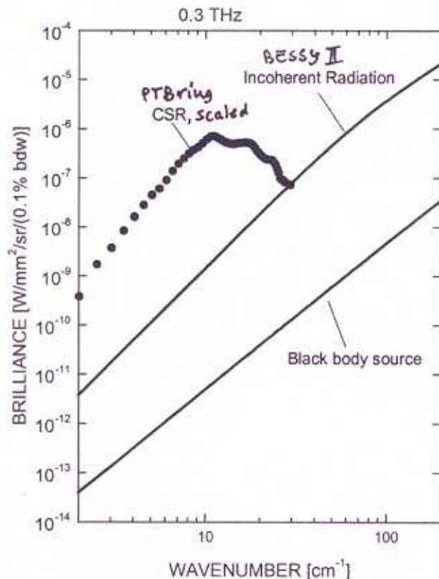
The expected CSR-brilliance for the PTB ring of the 5mA beam current, 40mradx60mrad. For comparison the incoherent intensity of the radiation of the BESSY II ring at 100 mA (incoherent radiation) and the radiation of a black body source is shown.
