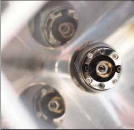
Flex structure for easy alignment of the \varnothing 4 mm sensor heads (image copyright ESRF).
