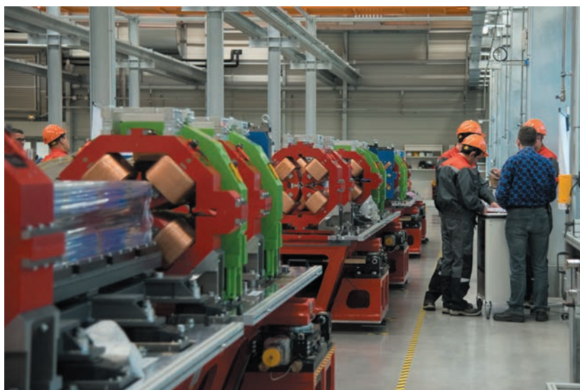
Fig. 4: The assembly line in ESRF 01. The assembly team is being supplemented by magnet and vacuum 'specialists' from Budker Institute of Nuclear Physics, Russia.
