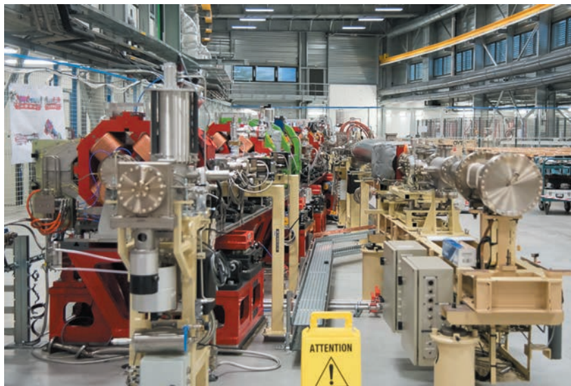
Fig. 2: The completed 'mock-up' of an EBS cell in the Chartreuse Hall.
