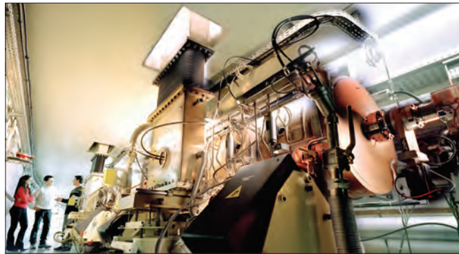
An RF cavity for accelerating electrons in the booster synchrotron.
