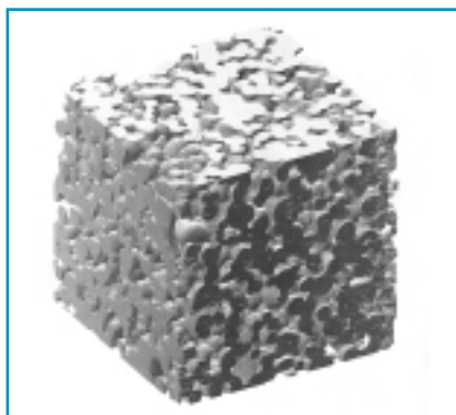
Fig. 2: 3D views of snow reconstructed from 1000 tomographic images. Image size is 600^3 voxels, voxel size is 10\ \mu\text{m} , exposure time 1s/view.
