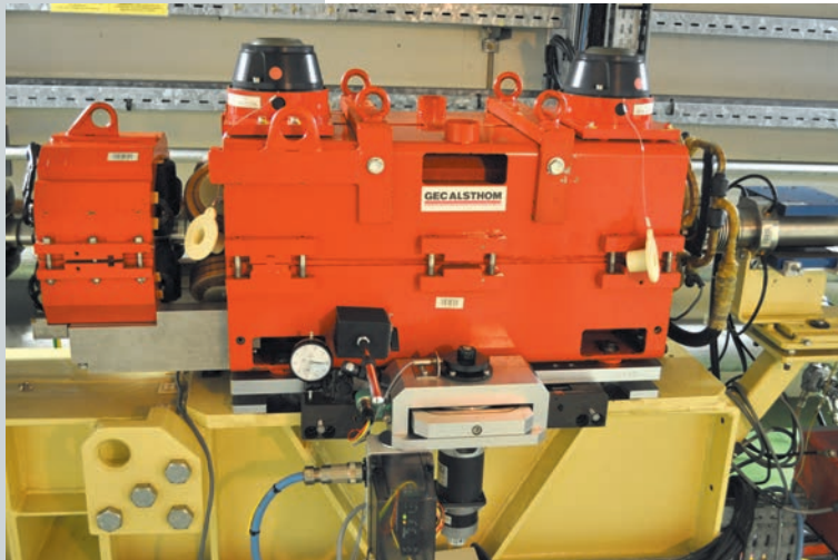
Fig. 166: Motorisation enabling a quadrupole in the booster to be displaced.
