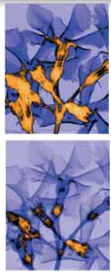
Images of a very low contrast object, taken with a) 200 electrons global threshold corresponding to 1 keV (LOW counter, all photons) b) at 6 keV threshold (1200 electrons). This image was taken in a single shot together with the previous one at 1 keV threshold
