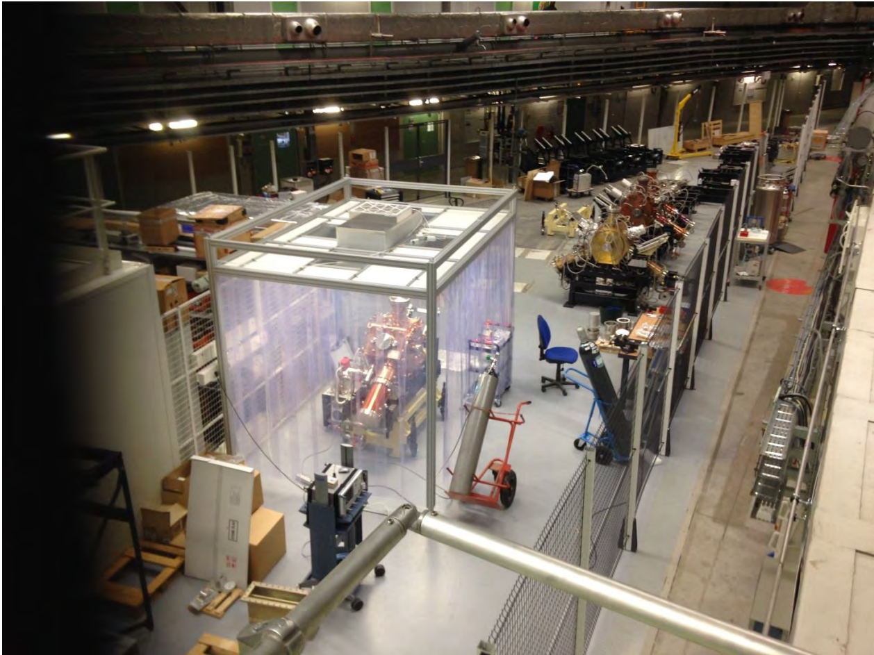
Figure 5.8: The cavity assembly area on ID08. In the foreground, the local clean room area for all UHV works, in the background, RF conditioned cavities and still empty girders.
