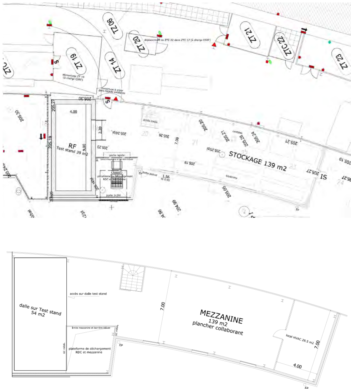
Figure 5.6: SRRF extension for a new RF power teststand and RF storage space – Pre-study June 2016-08-02.
